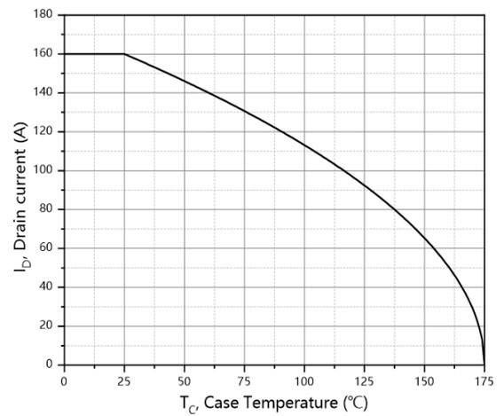
Figure 10. Drain current
