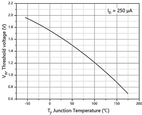
Figure 7. Threshold voltage
